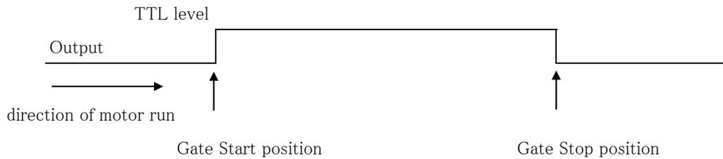
When you change Timing ready to # by **CHG** key, signal output "High" level between Gate Start position and Gate Stop position.
