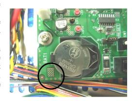
After replacing the battery, turn on the power of the main unit. "BATT EMPTY" is displayed when the power is turned on for the first time, but after that, the power is turned on again, and when the previous display disappears after the second time, the battery replacement is complete.
