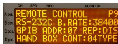
● 04TYPE Hand box controller (PM16-HDX 4 axis control)
