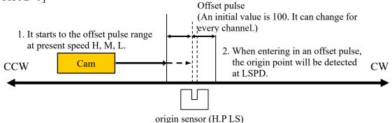
This way is used when the origin point information is memorized by the way previously described. The origin point is detected automatically based on the information memorized.
