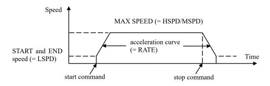
Acceleration operation is carried out until it will reach MSPD or HSPD by making LSPD into initial velocity, if a motion command is executed.
