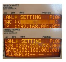
If change is completed, the SETUP button will be pushed, and escape from SETUP screen. The change will be reflected. Please check that communication is established by the "VER?" command etc.
