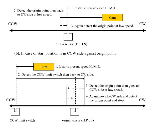
If a starting point sensor is detected, it will pass at first. And it will stop, if it passes completely, and it goes to the origin point by LSPD. Motor stopped suddenly, if the origin point sensor is detected from a direction opposite to the direction which started detection of the origin point. Then the position of pulse data is memorized and the direction approaching a sensor is also memorized.
