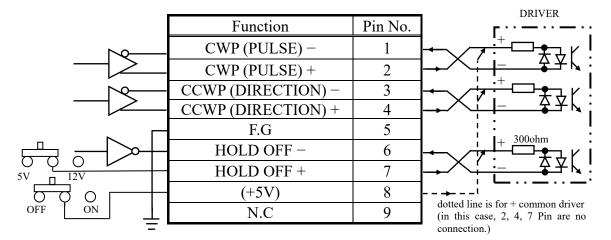
CWP (pins 1 and 2) and CCWP (pins 3 and 4) have a differential output of +5V-0V.
