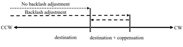
Ex.2) Move direction is CW and adjustment value is negative
