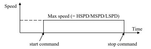
Motor drives at MAX speed as soon as drive execution, and stops immediately as soon as stop operation. Too fast drive speed causes motor step out. Low speed drive is always constant drive at all drive mode.
