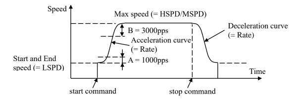
Although it is fundamentally the same as trapezoidal form acceleration drive, the velocity change at the time of acceleration and deceleration start and the time of acceleration and deceleration stop is performed according to S shaped form approximated to the parabola.
