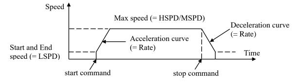
Acceleration operation is carried out until it will reach MSPD or HSPD by making LSPD into initial velocity, if a motion command is executed.
