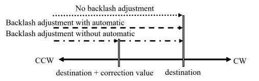
When the automatic adjustment is effective, backlash correction move is the same as no backlash correction. When the automatic adjustment is ineffective, as soon as the motor once stops at correction value, the motor drives to destination soon.
