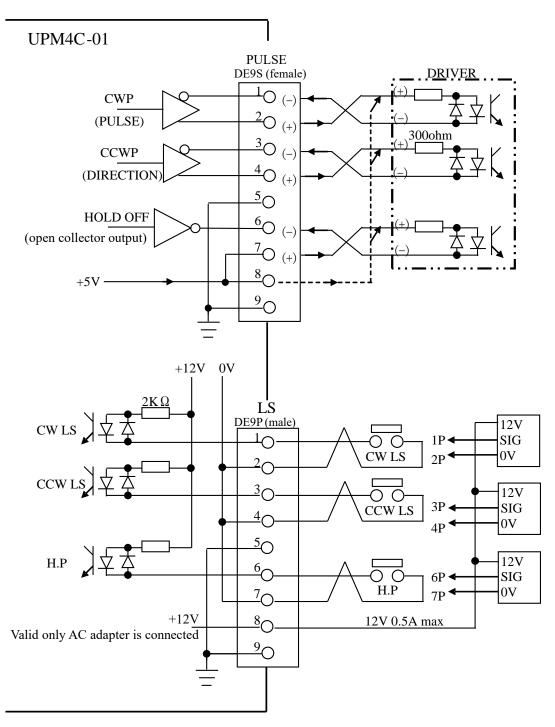
Connection cables are recommended to be shielded twist pair cable. (more than 0.2mm<sup>2</sup>)
